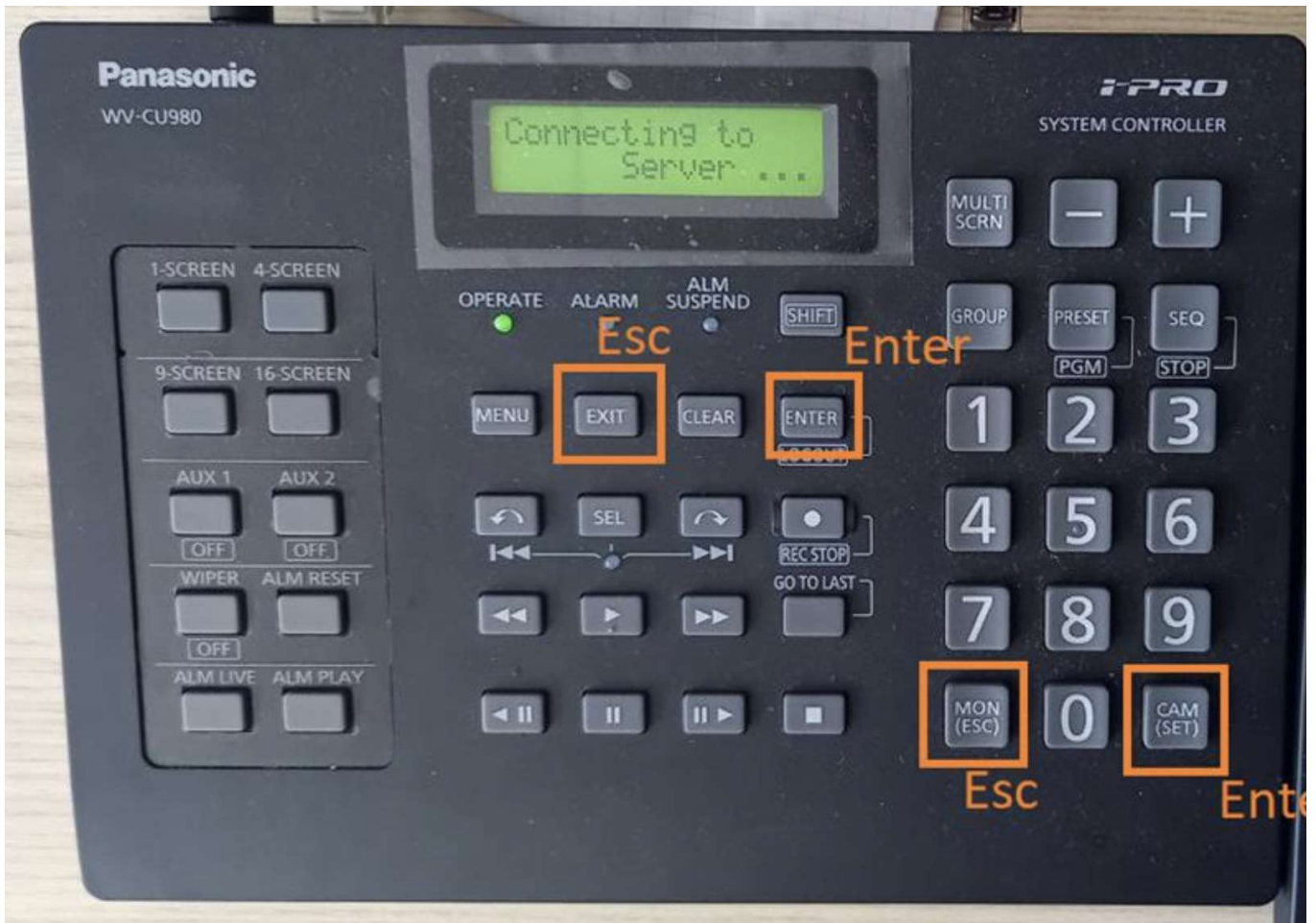
Mapping example: use the specified buttons to navigate in the Quick Popup dialog
