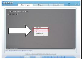
To modify sensor parameters, we must to change mode from standard to "**Debug Mode**" in configuration menu.
