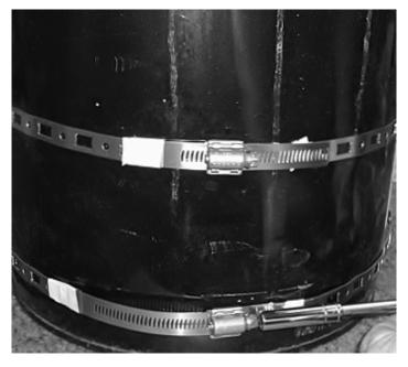
Check to make sure straps are securely tight and not twisted.
