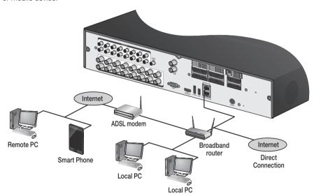
Connect the [ETHERNET] port in the rear panel to the router.
