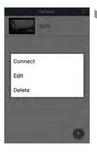
9 Select <Connect> and try to access. If connected successfully, you will see the screen as shown.
