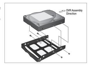
6. Push the bracket installed with new HDD back into the main unit until it is completely inserted.
