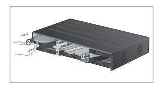
$\Bar{7}_{\star}$  Hold center of the ODD bracket's holder by your index finger and pull it.
