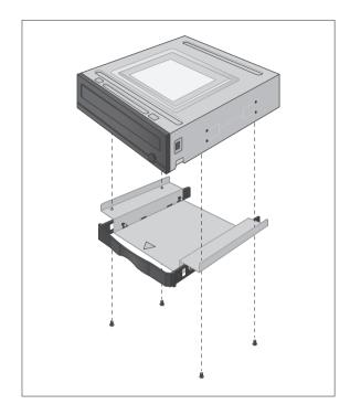
9 Insert the bracket with ODD into the main unit, push it until it's fully inserted.
