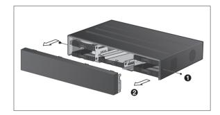
3. Hold the middle of HDD bracket's handle with index finger and pull it forward while sustaining the bracket handle with your thumb and middle finger as shown in the illustration.
