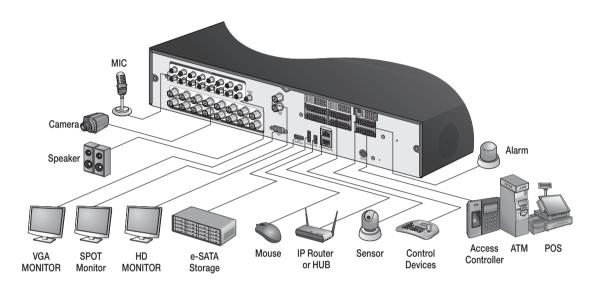
Since the cable quality may affect directly to the video quality depending on the distance between the camera and DVR, it is recommended to consult an authorized installer when installing the DVR.
