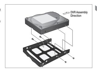
$\emph{6}_{\cdot}$  Push the bracket installed with new HDD back into the main unit until it is completely inserted.
