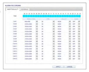
Complete setting the <SIZE/FPS/QUALITY/AUDIO> for the alarm recording as well as the <SCHEDULE>, and click <APPLY> to apply the changes.
